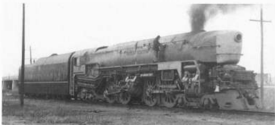
No. 5526, one of the 50 production T1's, still lacks some sheet-metal streamlining as its front-end throttle gets some attention at the Baldwin plant on November 30, 1945.
