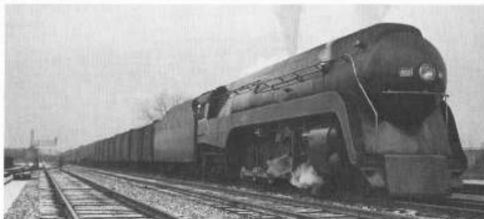
As it was working out the bugs in the T1 prototypes, PRR borrowed an N&W J for tests. The 4-8-4 (at Englewood), performed well, but PRR sent it home and ordered more T1's.
